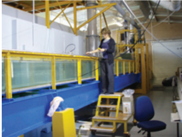
Figure 5.5 The 20 m recirculating flume with a water depth of 35 cm.
