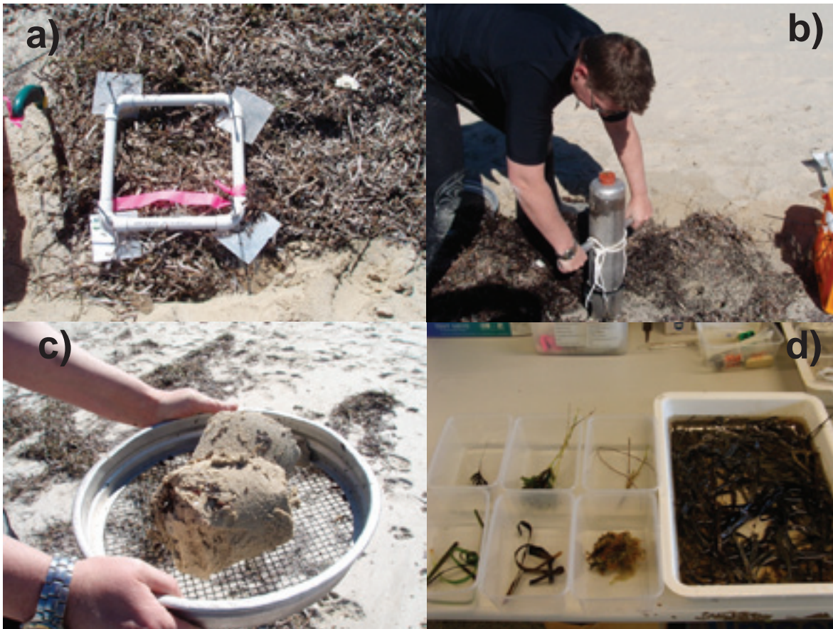
Figure 6.12 Methods to collect samples for above- and below-ground wrack composition. Above-ground samples were collected from within a 0.25 x 0.25 x 0.1 m area (a) and below-ground samples were taken with a core (b) and then sieved to remove sand (c). All samples were processed in the laboratory (d).
