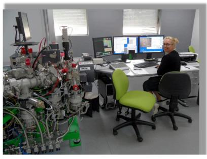
Analysing surface of a gold electrode with electrodeposited arsenic film using Secondary Ion Mass Spectrometer, SIMS, instrument at University of Western Sydney.
